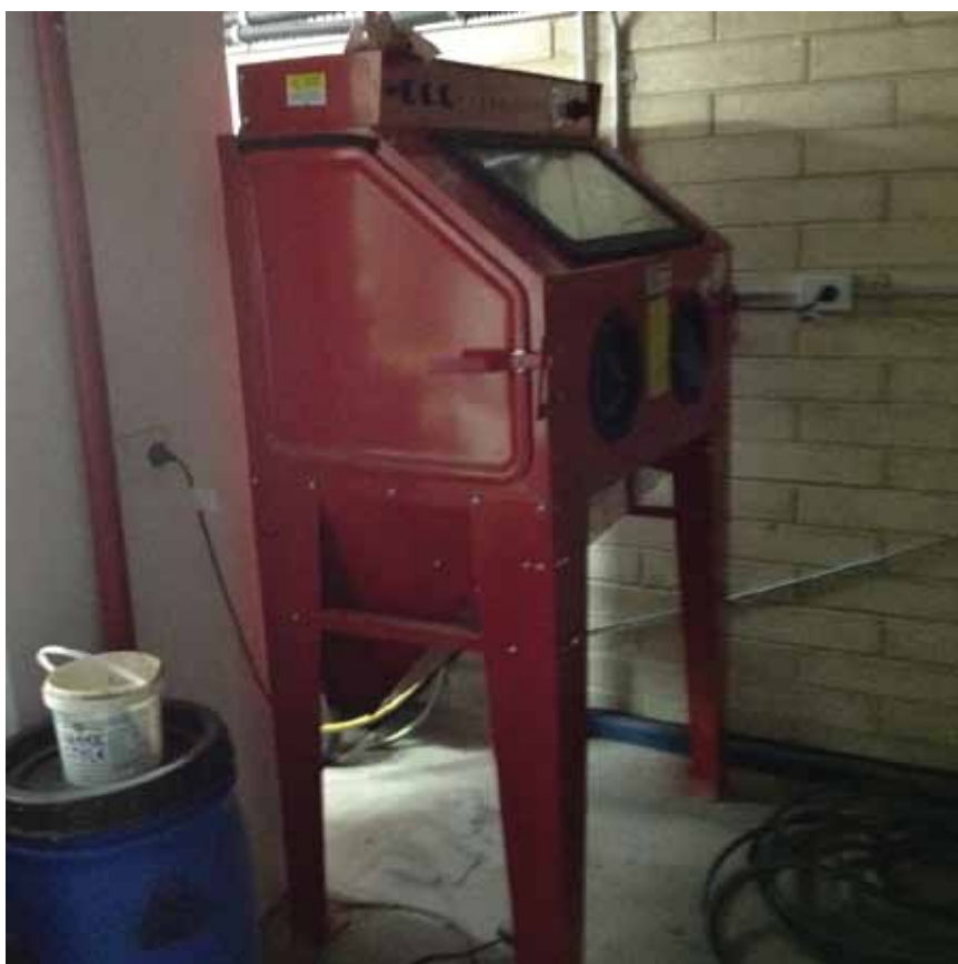
Image 1: Sandblaster in the council workshop
